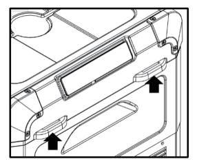
NOTE: Use all tie-down brackets when securing the fridge via the tie-down brackets.
